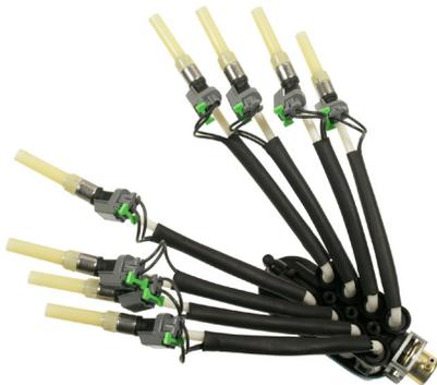
**Tech Tip:** For successful installation, lubricate injector tips and O-ring seals with transmission assembly gel, petroleum jelly, or even clean engine oil. Do not use silicone.
