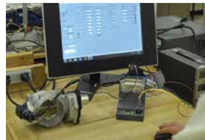
Tech Expert® engineer performing TPS output test
