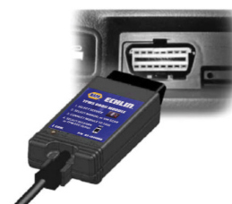
Connect tool to OBDII port
