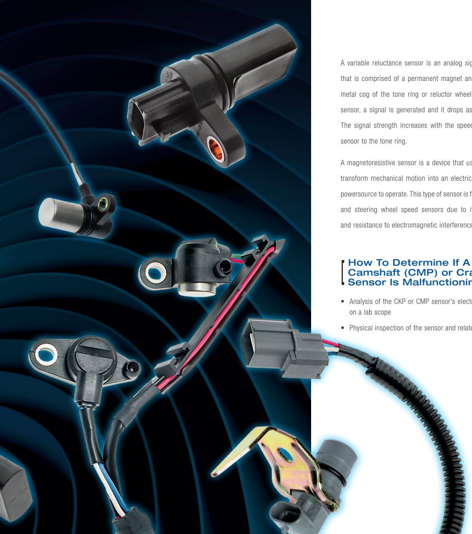
A variable reluctance sensor is an analog signal generating sensor that is comprised of a permanent magnet and a pole piece. As the metal cog of the tone ring or reluctor wheel passes the tip of the sensor, a signal is generated and it drops as the cog moves away. The signal strength increases with the speed and proximity of the
