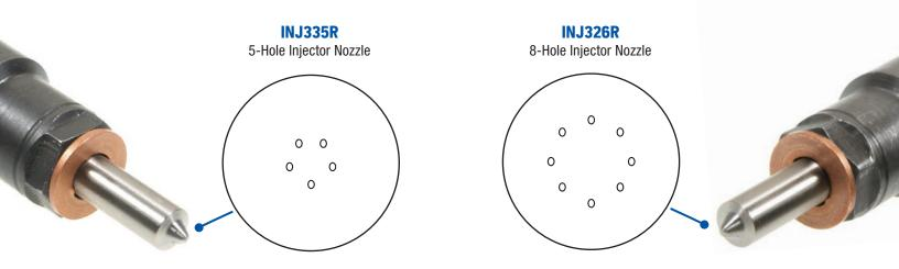
Installing the incorrect fuel injector on 2004 Dodge Cummins engines is a common error. Although the fuel injectors appear to be the same, they are not interchangeable. The NAPA® Echlin® INJ326R injector is designed with an 8-port injector nozzle and INJ335R features a 5-port injector nozzle.
