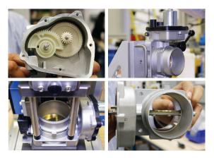
As an expert Electronic Throttle Body manufacturer, we maintain complete quality control throughout the entire manufacturing process. We assemble and calibrate the components matching OE output voltages to facilitate the relearn process.
