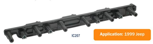
Caution: Inspect the ignition coil bar for cracks and any signs of arcing. Arcing at the secondary end will cause the rubber boots to carbonize which can cause the coil to fail. Replace coil bar if any cracks or signs of arcing are found. Primary specs only .71 - .88 Ohms
