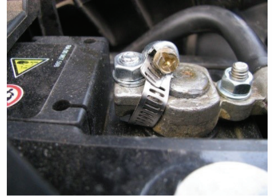
Temporary Hose Clamp Repair
