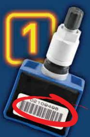
Locate the ID on the original sensor and type it into the cloning tool.
