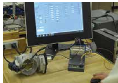
Tech Expert® engineer performing TPS output test
