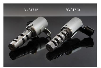
Years: 2001-2007 Make: Toyota Engines: 3.0L and 3.3L Common DTC: P1354 Symptoms: Rough idle Solution: Maintain regular engine oil change intervals. When replacing the solenoids, replace the engine oil and filter. Parts for the job: VVS1712 and VVS1713
