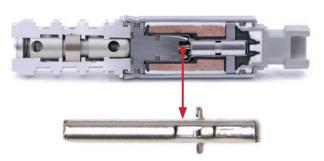
Uses a soft aluminum internal shaft which can deform over time and alter the timing of the valves
