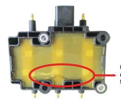
OE epoxy cracks after temperature test
