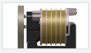
OE coil uses 5 bobbin segments with 27 kV (5.4 kV per segment)
