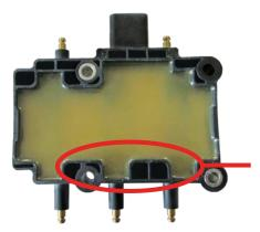
No cracks after temperature test
