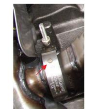
6. Install LH and RH exhaust inlet pipe-to-exhaust manifold nuts. Alternate tighten the bolts on each side of the engine to draw inlet pipes equally to each exhaust manifold flange. Note: Gap between pipe flange and exhaust manifold should be even for both exhaust connections on the engine.
