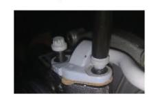
10. Position oil supply line with new gasket, then install original
