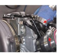
11. Install inlet & outlet air hoses to the turbocharger compresso
