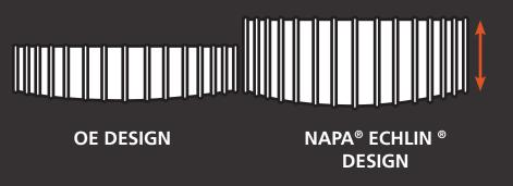
After studying the failed **OE unit, we increased** face width on the NAPA® Echlin<sup>®</sup> gear by 17% to reduce stress on the gear teeth
