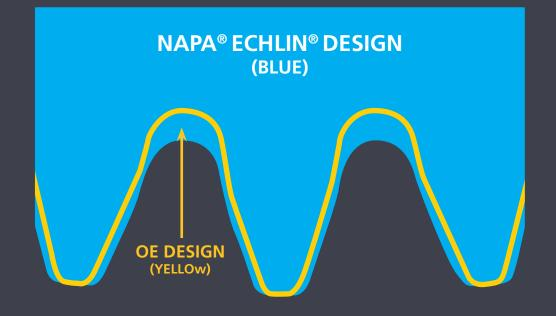
**NAPA<sup>®</sup> Echlin<sup>®</sup> engineers** improved the gear stiffness by increasing tooth thickness and decreasing overall tooth length to build a more durable gear
