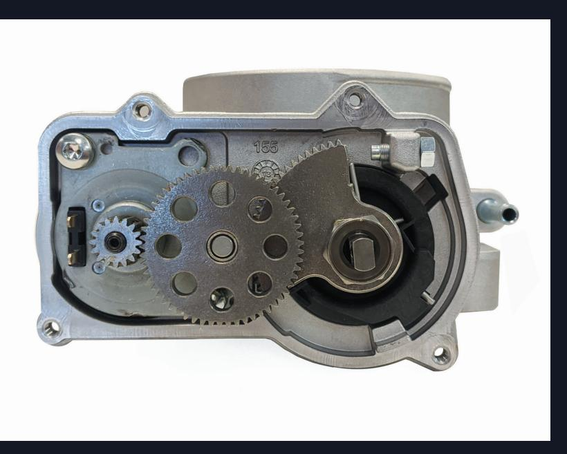
Even after 45 days of endurance testing, our ETB was intact and fully operational
