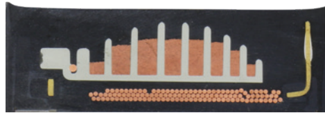
The OE coil has 8 bobbin sections
